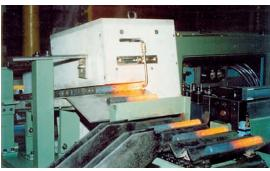
Forging heating is very important process in forging production. The induction heating and heating with gas are the main method in forging industry. How to increase heating efficiency, uniform and temperature accuracy are the vital issues. That large gas furnace with regenerator burning system installed has brought a significant energy saving, and improved the emission, but the energy utilization is still expected to be improved.
